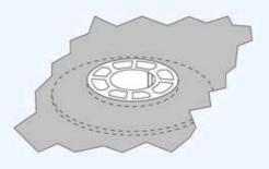
$3^{\mathrm{Push}}$  the lower washer flange up through hole from the underside of cover.
