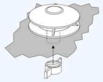
$\mathbf{5}^{\text{Then screw}}$  the wingnut on tightly from the underside of the cover.
