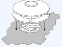
4 Push the cap down through the hole from the top side of the cover.
