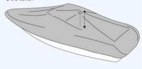
6 Push pole into vent hole from the underside of cover and adjust cover for proper height. Use the knob to lock pole at proper height so that no dips where water could pool are evident.
