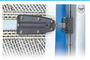
Series 35 luff boxes connect to the slide with a cleverly concealed M10 nut that provides a solid connection and full lay flat
