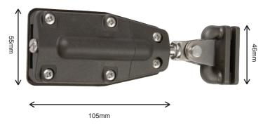
Luff boxes. Series 25 luff boxes connect to the slide with a cleverly concealed M10 connecting thread, allowing compatibility with Sailman 3000, 3500 and 4000 slides, as well as most other slide systems. The cover plate design allows easy installation and removal of battens, while the body remains fastened to the sail. Sailman 25 series luff box has been designed for small boat applications, such as cruising sloops, up to about 30ft.
