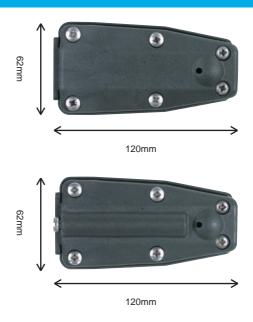
Luff boxes. Series 35 luff boxes connect to the slide with a cleverly concealed M10 nut that provides a solid connection and full lay flat rotation of the batten. The long housing ensures the batten remains in place while the supplied batten guides allow the choice of either 10mm round or 30mm flat battens and provide the additional benefit of an integral screw tension adjusting system.
